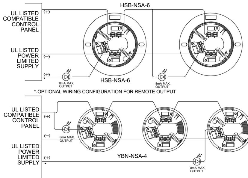
**NOTE:** Fire alarm control panel compatibility is required for DCP products. DCP communications protocol allows system components (DCP sensors AIE-EA, ALG-V, ACA-V, ACC-V, ALK-V, ALN-V, ATJEA and ATG-EA, bases and modules) to be used concurrently on a system's SLC (Signaling Line Circuit).
