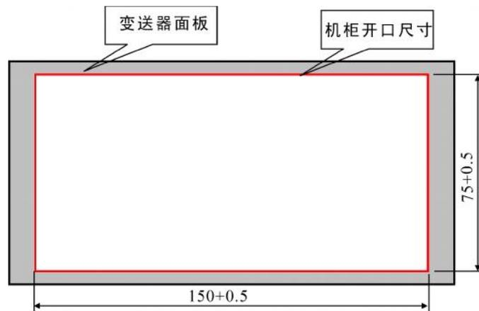
Before installation, please remove the mandrel on both sides of the casing, and then weighing terminal into the cabinet, the two ejector fixed on both sides of the weighing terminal, requiring top tight control housing to ensure secure installation.
